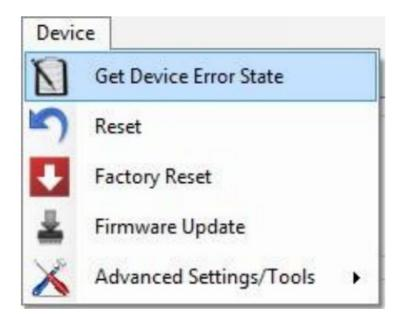
The SFC5xxx has an internal error status register. You can show the "Device Error State" window by clicking on the menu item Device → Get Device Error State.
