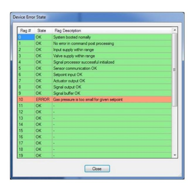
• If e.g. gas supply pressure drops down and MFC can't reach the setpoint, the correspondent error status will turn red in the "Device Error State" list.
