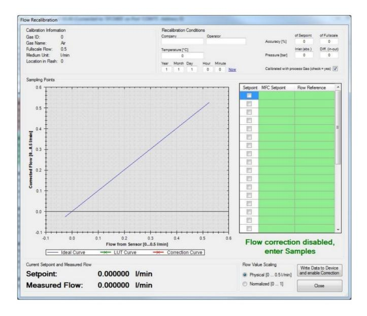
If the sensor has become inaccurate due to changes in environmental conditions or aging, the sensor readings can be corrected with an additional lookup table. With this tool you can find, set and verify the points for this lookup table. Instructions are described below in the document.
