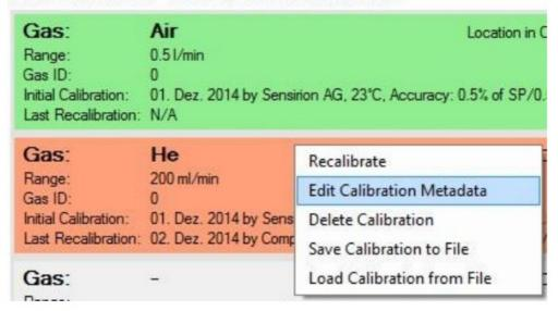
• In this window you can change the metadata of a given calibration.
