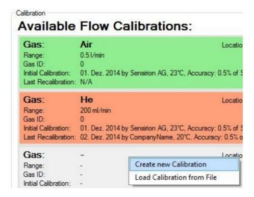
• Select an existing calibration with similar gas characteristics from the drop-down menu.
