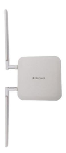
GWX is a gateway device meant to be used with wireless sensors. GWX uses 868 MHz (EU only) and/or 2.4 GHz proprietary radio to advertise itself to nearby sensor devices so they can connect and send their measurement data. GWX then transmits the data to Sensire Cloud via LTE/3G/2G connection. GWX also includes NFC that can be used to configure and debug the device using a mobile device and Sensire provided app. GWX can also configure sensor devices using the NFC.
