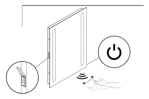
Caution: To avoid interference, the sensor must be placed a minimum of 150mm away from any object/surface
