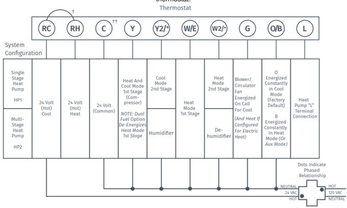
†Internal jumper between RC and RH, located on the back of the thermostat. Common connection required on Heat-only, Cool-only, or Heat Pump systems.
