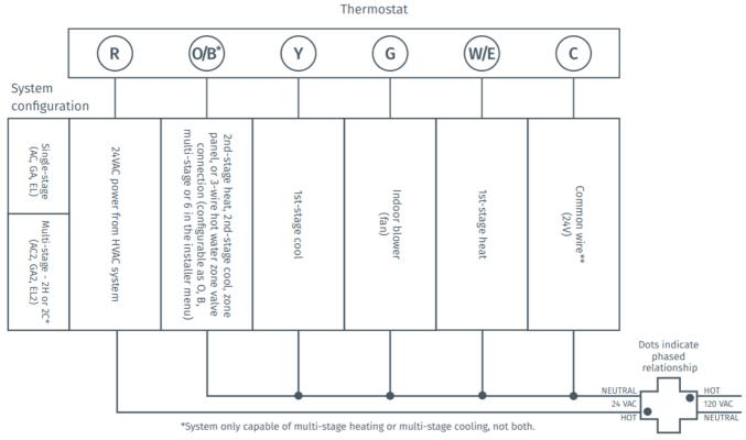
$\ensuremath{^{**}\text{Common}}$  connection required on heat-only, cool-only or heat pump systems.
