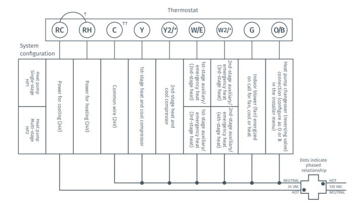
† Internal jumper between RC and RH, located on back of thermostat.
