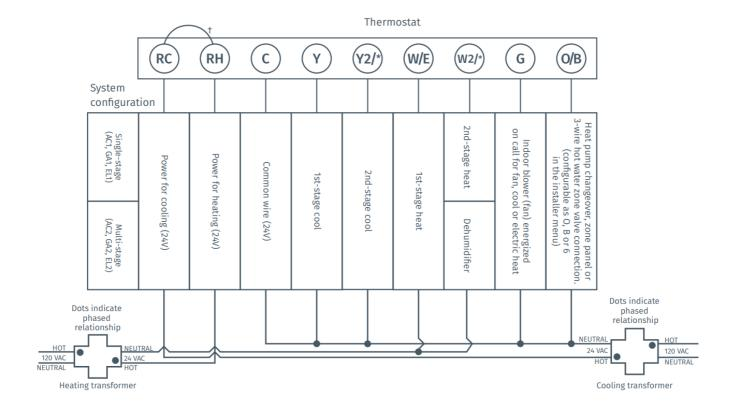
Two transformers systems (separate RC and RH wires), clip internal RC/RH jumper, located on back of thermostat.
