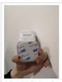
Paste 3M adhesive to the bottom of the equipment
