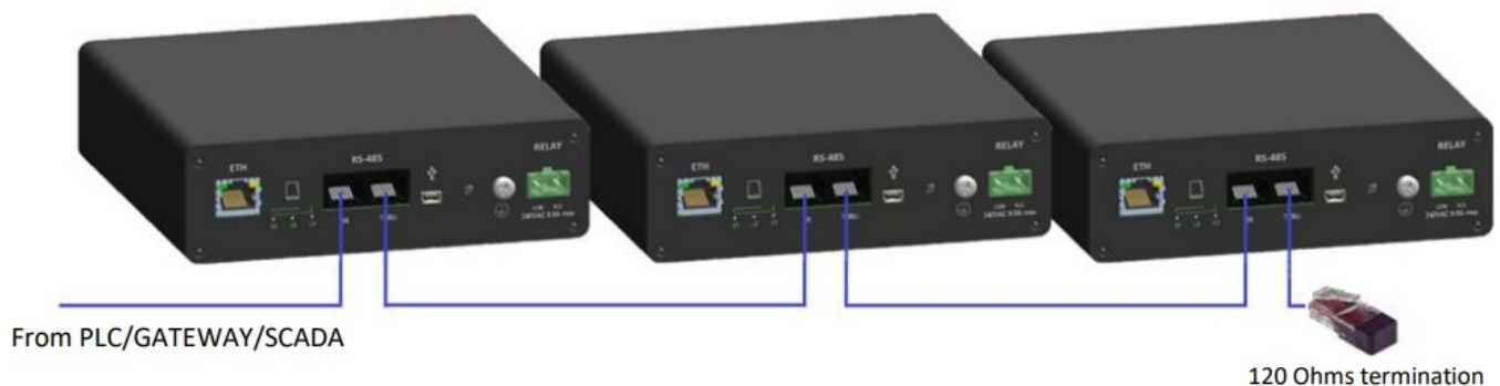
Figure 16: RS485 daisy chaining
