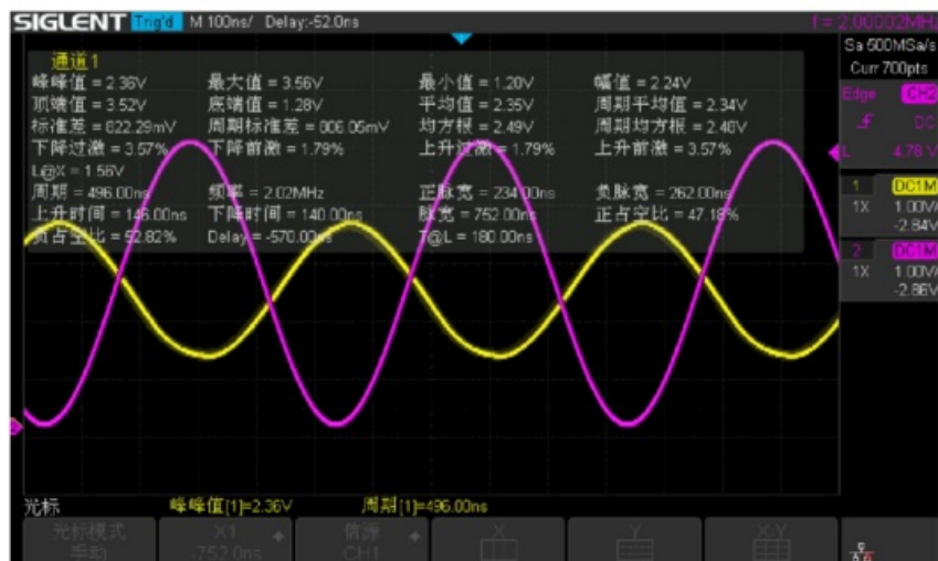
Figure10 Modulation Bandwidth Test Diagram (Purple: A 2 MHz sinusoidal signal input ranging from 0V to 5V, tested with a 10 Ohm load; Yellow: The curve representing the actual current response after a 3dB drop)
