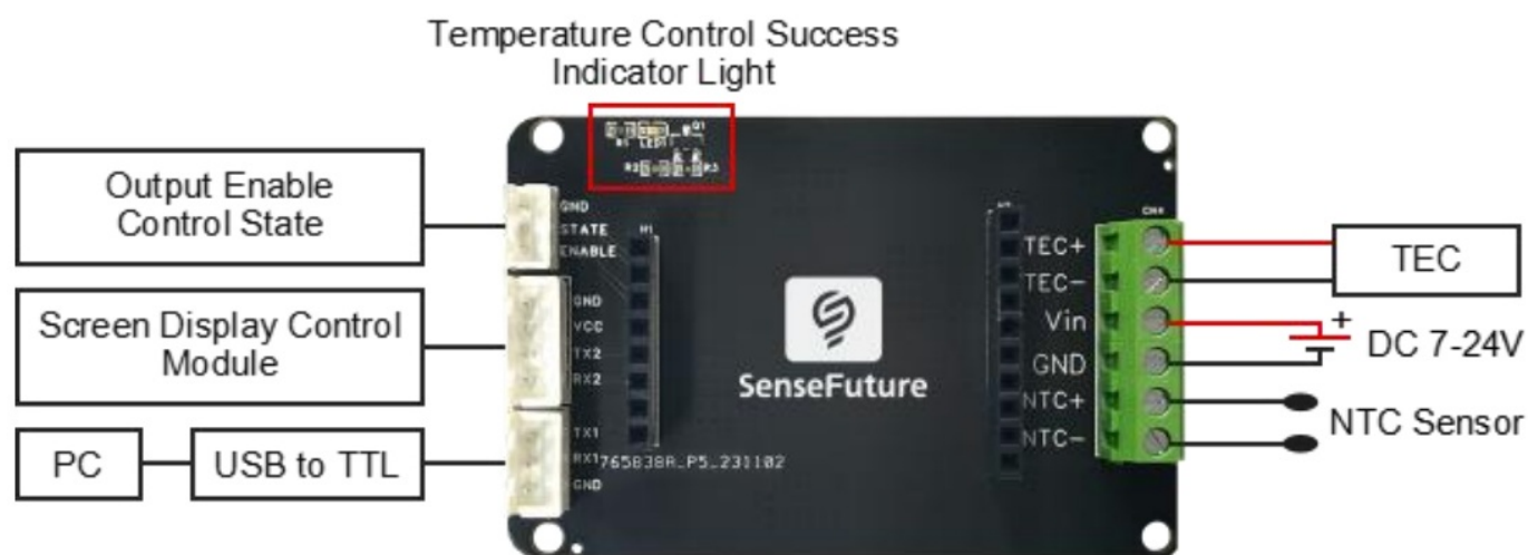
Figure3 TEC103/TEC103L Adapter Board Wiring Diagram
