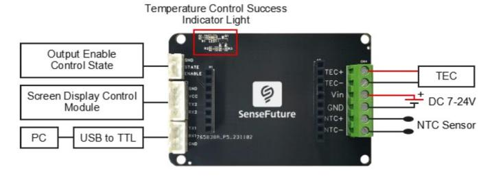
Figure3 TEC103/TEC103L Adapter Board Wiring Diagram
