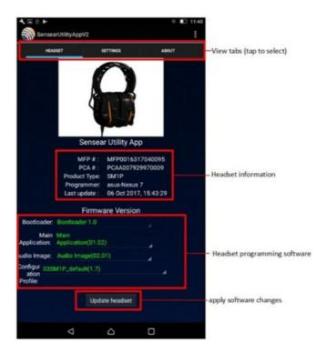
The device tab displays device information such as product type, MFP numbers, etc. It also displays the currently programmed software versions. The different firmware can be programmed from this tab. Note that firmware is specific to a product or a family of products.
