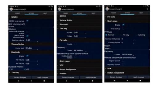
The "Settings" tab outlines the configurable features that are displayed for configuration. The settings are a way of customizing the configuration profile. This allows the app to disable/enable some features, set levels, program frequencies, etc. Depending on which headset is connected, only applicable options should be displayed.
