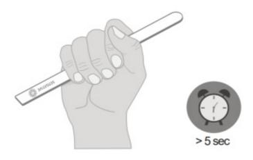
You may verify that your Z-Wave controller shows Strips Drip reporting correctly by holding it firmly according to the illustration above for >5 seconds. Strips Drip will sense the moisture level and send a leakage alarm. After removing your hand, the water leakage alarm should disappear.
