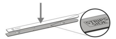
Remove the protective tape from Strips Drip adhesive. Mount Strips Drip on the marked "Strips Side" of the mounting plate as illustrated above.
