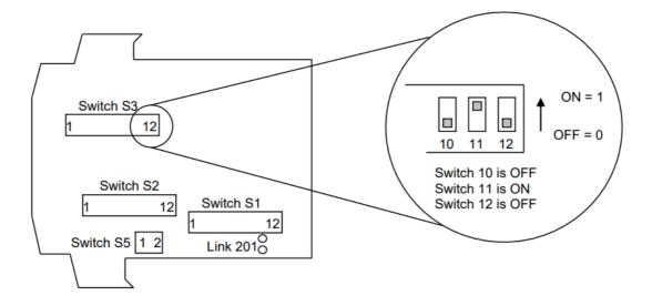
Switch S1 and S2 configures input 1 type, S1, and S5 configure input 2 types, and S3 configures the output type and function. Link 201 should be fitted for a 3-wire potentiometer on input 1. The switch settings are explained in the next few pages. The diagrams refer to switch positions 0 and 1, with 0 being OFF and 1 being ON. This is illustrated in the picture above.
