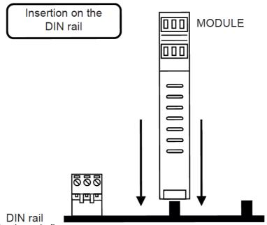
Insertion in the DIN rail As shown in figure:
