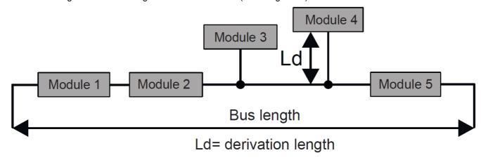
For maximum performance, it is recommended to use special shielded cables, such as BELDEN 9841.
