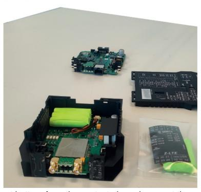
6. Disconnect the spent battery from the contact pin and connect the new battery to the contact pin.
