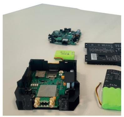
7. Connect the new battery to the contact pin. Reposition the new battery to its original location and close the product.
