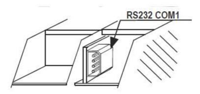
The Z-PASS1 has serial RS232 or RS485 COM1 port on the removable 4 pin contacts connector. The cable length for the RS232 interface must be less than 3 meters.
