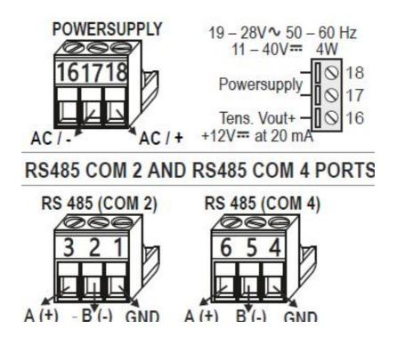
In addition to the IDC10 connector, power supply can also be supplied by terminals 17 and 18.
