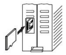
**LOT FOR MICRO SD CARD:** The Z-PASS1 has a slot for micro SD card placed on the side of the case. Before pushing the micro SD or micro SHDC in this slot, please be sure that the SIM card golden contacts are facing towards left (as in the picture on side).
