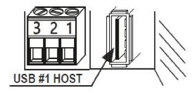
**USB #1 HOST PORT:** The Z-PASS1 has a USB HOST type A connector, here you can connect a USB memory stick for firmware upgrading. Available current: 100 mA MAX.
