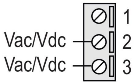
Terminals 2 and 3 can be used to provide the module with power supply as an alternative to the connection using the Z-PC-DINx bus.
