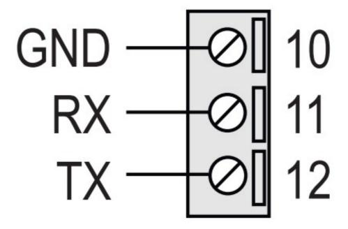
The module has a serial port that can be configured with the SW2 switch.
