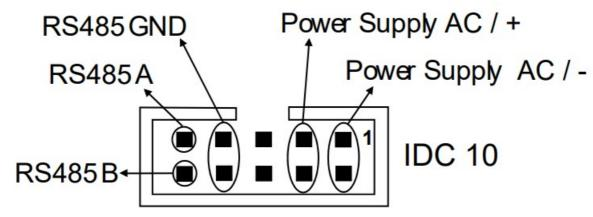
The illustration shows the meanings of the various IDC10 connector pins if signals are to be sent via them directly.
