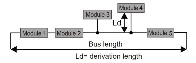
For maximum performance, it is recommended to use special shielded cables, such as BELDEN 9841.
