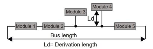
For maximum performance, it is recommended to use special shielded cables manufactured specifically for RS485 communication.
