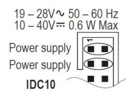
Connect the IDC10 rear connector to provide power supply to module.
