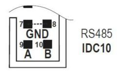
Connection for RS485 communication with the Modbus master system through Z-PC-DINAL2-17.5 accessory. **Note:** the indication of the RS485 connection polarity is not standardised and in some masters may be inverted
