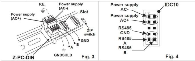
In case of Z-PC-DINAL2-17,5 accessory use, the signals may be provided by terminal blocks. The figure shows the meaning of terminals and the position of DIP-switch (present on each DIN rail supports) for network termination (not used in case of Modbus network).
