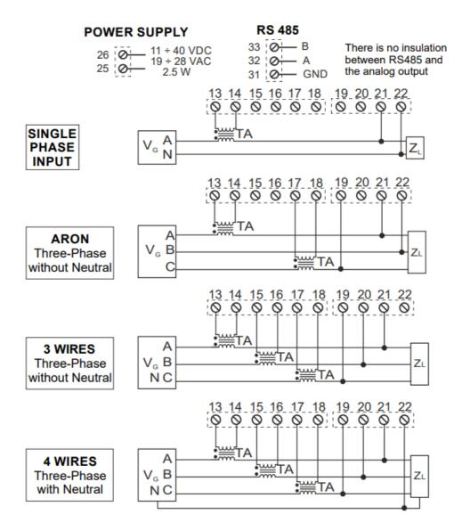
**Note:** You can't connect the secondary of any CTs to the Earth. Terminals 14, 16 18 and 22 are internally connected.
