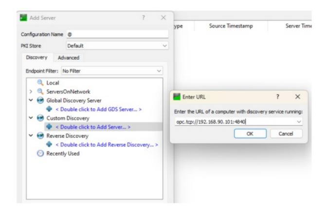
By pressing OK the server is added to the list, select the desired encryption (None in this example):
