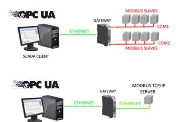
The Gateway, on the field side, works as a Modbus master / Modbus Client device and on the other side as an IEC 61850 server via Ethernet.
