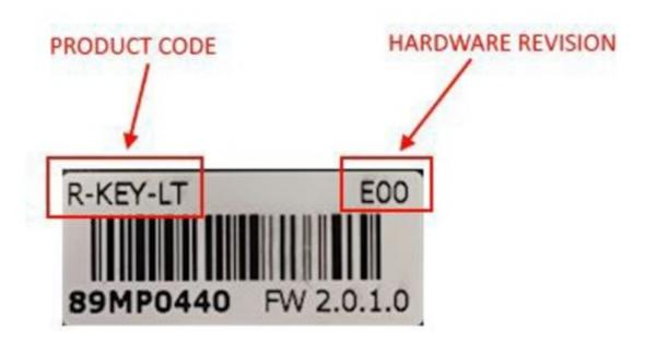
The label also shows the firmware revision present in the device (in this case 2.0.1.0) at the time of sale, the hardware revision (in this case) is E00.
