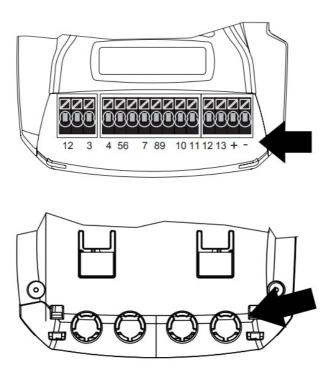
MyAlarm2 has a terminal block inside its enclosure. To access the internal terminal block of the device, unscrew the screw at the centre of the black cover positioned at the bottom of the enclosure and lift up. In the side figure, the cover has been removed.
