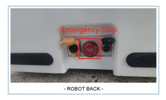
To release the emergency stop state of the robot, please twist in the direction of the button (clockwise)until the emergency stop springs back, then you can select continue/cancel the current task on the screen.
