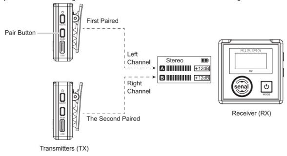
If the transmitter is disconnected, re-pair it to the receiver by pressing and holding the Pair button.
