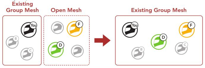
1. One (You) of the current users in the Existing Group Mesh and new users (D and F) in Open Mesh enter into Mesh Grouping to join the Existing Group Mesh.
