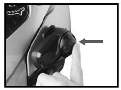
• To track forward or track back, rotate while pressing the Jog Dial clockwise or counter clockwise.
