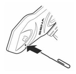
If the 10R is not working properly for any reason, reset by gently pushing the pin-hole reset button located below the (+) button.
