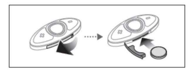
To begin using the RC3, take off the plastic cover in the battery slot. When closing the battery slot, insert both ends of the rubber first. To remove the battery, insert a paper clip through the Battery Release Hole.
