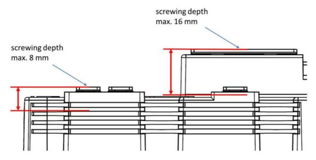
When using an electrical screwdriver, screwing speed has to be limited to a maximum of 300 rpm and soft torque limitation is recommended. SEMIKRON do NOT recommend pneumatic screwdrivers due to clutch behavior with torque overshoots.
