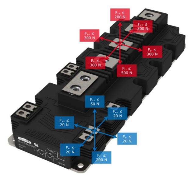
It is recommended to have a construction which leaves the power and auxiliary terminals permanently free of mechanical stress during operation. To achieve this in a wide temperature range it is advised to add suitable spacers. It must be ensured that the direction of the force always acts towards the direction of the base plate. Static forces in other directions as well as exposure to vibration and / or thermal expansion should be avoided.
