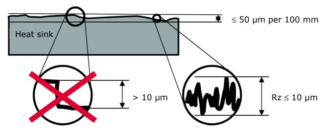
The condition of the heat sink contact area should not exceed the values in Table 5, otherwise inhomogeneous heat dissipation can lead to partial overheating of the semiconductors.
