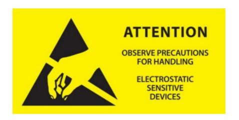
All staff should be trained for correct ESD handling. The user must observe all precautions in order to avoid electrostatic discharge during handling, movement and packing of these components.
