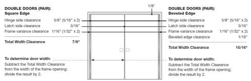
**NOTE:** For double-door entrances with a mullion between the pair of doors, calculate each door width using the Single Door clearances. For double-door entrances with a mullion behind the pair of doors, calculate each door width using the Double Doors clearances.
