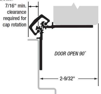
**FINISHES:** All SL31 hinges are stocked in Clear and Dark Bronze anodized aluminum. Custom anodized or painted finishes are available. Product painted or anodized in the field voids the SELECT hinge warranty. **CLOSERS:** Conventional overhead surface, concealed sliding arm overhead or floor closers may be used with SELECT hinges. Pivot-type floor closers (with a fixed, conflicting center pivot) must be replaced.
