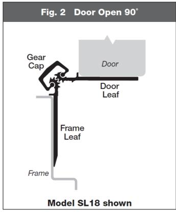
making sure frame leaf alignment flange is tight against frame face.
