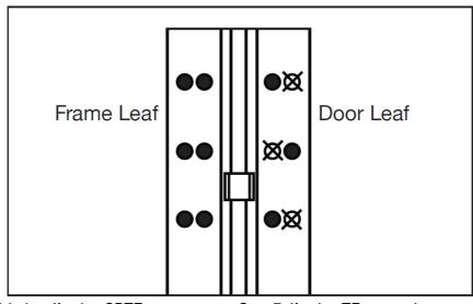
6. Mark (or centerpunch) holes. If using SDTF screws, go to Step 7. If using TF or wood screws, drill holes at
