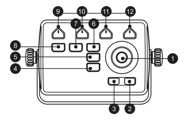
1. The joystick can move the cursor around the map or through menu items. Press [UP], [DOWN], [LEFT] or [RIGHT].
