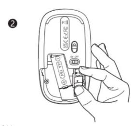
3. Turn the power switch to ON.
