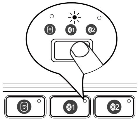
3. Hold and press the BT1 button for 3.5s until the white indicator light blinks quickly, indicates your keyboard has entered into Pairing status.
