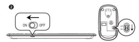
Turn the power switch to ON.
