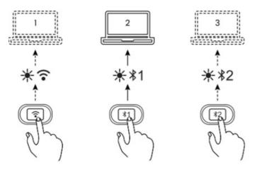
After ( are connected, single press the channel button on the keyboard, easily switch between multiple devices.
