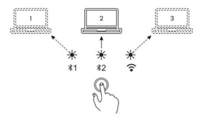
After \*1 \*2 \rightarrow are connected, single press the channel switch button on the bottom of the mouse, easily switch between multiple devices.
