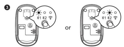
3. Press the channel switch button until the \*1/\*2 channel indicator light is on, and the mouse enters the Bluetooth channel. Long press the channel switch button for 3~5 seconds until the indicator light flashes quickly, and the mouse enters Bluetooth
