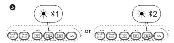
3. Press \*1 / \*2 channel button, and the \*1 / \*2 corresponding indicator light is on, the keyboard enters the Bluetooth channel. Long Press this selected channel button for 3~5 seconds until the corresponding indicator light flashes quickly, and the keyboard enters Bluetooth paring mode.
