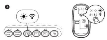
3. Press the channel button, and the channel indicator light is on, the keyboard enters the 2.4G USB channel.
