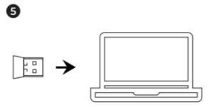
5. Plug the USB receiver into the USB port of the computer, the keyboard and mouse will connect automatically.
