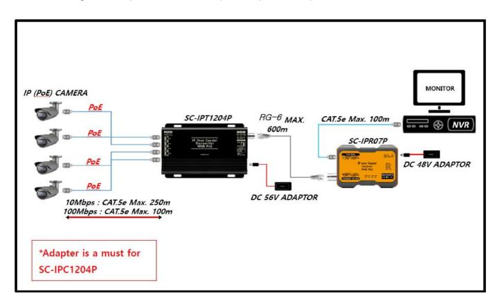
In case of using 8CH transmission configuration
