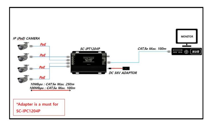
In case of using with EoC(Ethernet over Coax.) device (SC-IPR07P)
