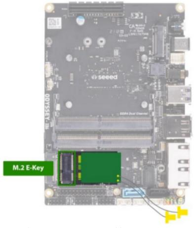
**Note:** reServer is shipped with two 2.4/5GHz WiFi Antennas, you can attach the antenna to the adapter which connects with the antenna cable of the WiFi module inside the reServer to achieve
