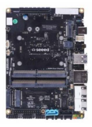
ODYSSEY X86 v2 board powered by the latest Intel® Core™ 11th Gen. processor and Intel® UHD Graphics or Intel® Iris Xe Graphics, which delivers high CPU and AI performance for various applications. It has two high-speed 2.5-Gigabit Ethernet ports and supports hybrid connectivity including, BLE and WIFI. Meanwhile.
