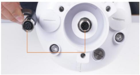
3. Plugin the cable and tighten it clockwise
