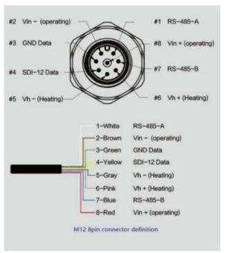
1. Wire sequence of ONE Compact Weather Station Sensor:
