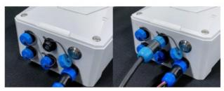
When connecting the aviation connectors, align the widest groove on the male head to the position of the flat head, insert and tighten
