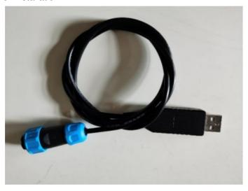
The aviation connect (blue part) is connected to the power port (B6) of Sensor Hub Data Logger and the USB port is connected to the computer.
