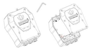
2. SwipedownwardtoopentheSIMcardsocket,insert the MicroSIMcardandswipeupwardtolocktheSIMcardsocket. Makesureitisinstalledcorrectlyandclosethelidwiththescrews.
