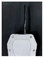
**Note:** Do NOT connect the power supply when installing the antenna, as this may cause damage to the antenna circuit!
