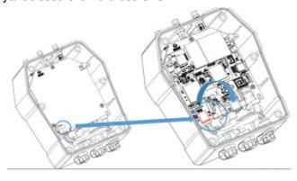
**Note:** When installing the cover screws, be sure to lock the screws tight, or it may affect the water resistance of the device!
