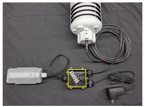
5. Tighten the screws and screw caps to check the waterproofing. If the wire diameter is too thin, add waterproof tape for winding
