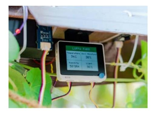
**Meilily Li** and **Lakshantha Dissanayake** designed a solar-powered, IoT-based farming system that monitors temperature, humidity, soil moisture, and light levels. This system was installed at the Luffa farm.
