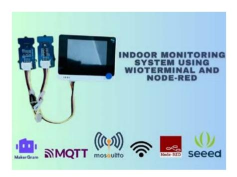
**Muhammed Zain** and **Fasna C** created an Indoor Monitoring System using the Wio Terminal, Grove-Temperature & Humidity Sensor (SHT40), and Grove-VOC and eCO2 Gas Sensor (SGP30).
