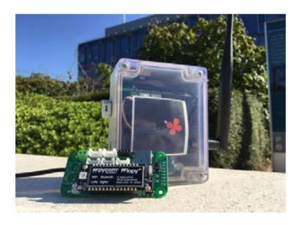
PyonAir, shared by **Hazel M.**, is a low-cost and open-source system for monitoring local air pollution levels-specifically, particulate matter, and it transmits data over both LoRa and WiFi.
