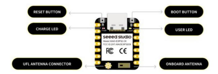
This new XIAO is equipped with a high-performance onboard ceramic antenna with up to 80m BLE/Wi-Fi range, while it also reserves an interface for an external UFL antenna. At the same time, it also comes with an optimized power consumption management. Featuring four power modes and an onboard lithium battery charging management circuit, it works in the Deep Sleep mode with a current as low as 15 μA, making it an excellent fit for remote, battery-powered applications.
