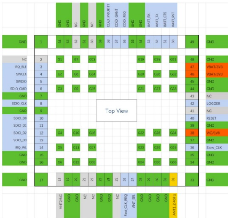
Figure 2-3. BM3301-1313 Module Pin arrangement
