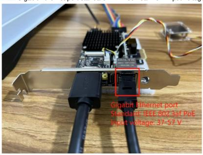
When using Po E power supply, there is no need to connect the **PWR-IN** port.
