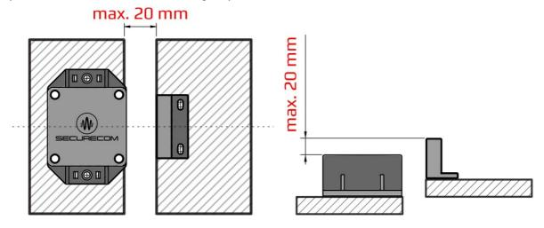
Moving the magnet closer or further away from the device, i.e. opening or closing the gate will cause the blue LED on the unit to flash. (this is visible under the cover plate in low light conditions
