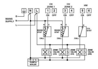
ChannelPlus H37XL Series 2 Controlling 3 x two port spring return zone valves via RoomStat and CylinderStat giving independent control of Hot water and two zones of Heating.
