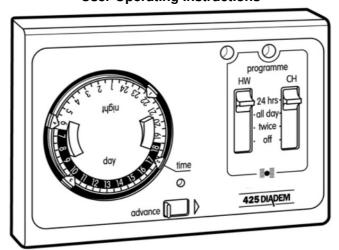
The 425 Tiara and Diadem programmers are 2 circuit central heating and hot water programmers able to switch ON and OFF twice every 24 hours. An advance switch is provided to make temporary overrides to the ON or OFF periods and a selector switch gives a further choice of programmes.
