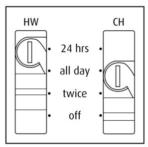
**Gravity** – On this type of system it is possible to have hot water without central heating, but not central heating without hot water. In this case, the installer would have interlocked the select switches as illustrated.
