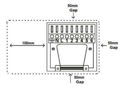
The backplate should be fitted with the wiring terminals located at the top and in a position that allows the relevant clearances around the programmer (see diagram)
