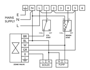
425 Diadem/Tiara controlling gravity hot water with pumped heating via room stat and cylinder stat 425 Diadem/Tiara controlling gravity hot water with pumped heating using a 2 port spring return valve with changeover auxiliary switch on the hot water circuit
