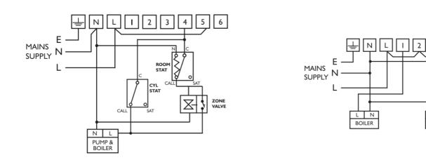
425 Coronet controlling fully pumped system via room stat, cylinder stat and using a 2 port spring return valve with auxiliary switch on the heating circuit
