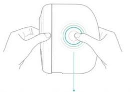
Press buttons on both sides, and pull out the back cover.
