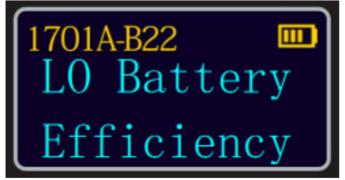
Step 6: Press Menu/OK to change to high or low battery efficiency.
