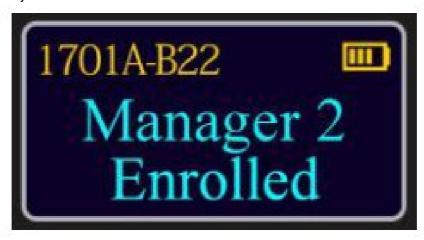
The new code is now enrolled and available to be used to open the lock.
