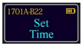
Step 5: Each of the elements of the date and time will flash when it is available to be set. Use the "▼"or "▲" to scroll to the correct value and Press OK to move to the next element.
