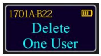
Step 6: Press the "Menu/OK" button first, then select the user to be deleted through the "▼" or "▲" button, and finally press the "Menu/OK" button to prompt the screen:
