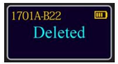
**Note:** If this operation is performed, the smartphone app will not be able to open the lock. If the operation, such as opening the lock through the app is required, it needs to be paired again.
