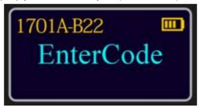
Step 4: The LCD screen will display a key Code. Record this number and call an authorized SECURAM Recovery Center or SECURAM Tech Support at 1-805-988-8088 for an Authorization Code. (This code remains valid for a period of 20 minutes only).
