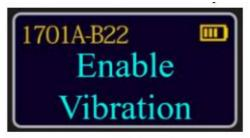
If the screen shows "Disable Vibration": The Vibration Alert is enabled. When vibration is sensed, the display will show Vibration Alert and the buzzer will sound. A notification will be sent to the paired smartphone app. If the screen shows "Enable Vibration": The Vibration Alert is disabled: no alert is displayed.
