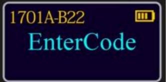
Step 4: The LCD screen will display a key Code. Record this number and call an authorized SECURAM Recovery Center or SECURAM Tech Support at 1-805-988-8088 for an Authorization Code. (This code remains valid for a period of 20 minutes only).
